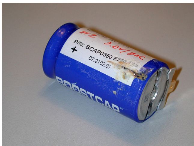
Fig. 10. A BCAP0350 capacitor (cell 2) tested at 3.0 V and 70 °C after safety valve opening after 200 h.
